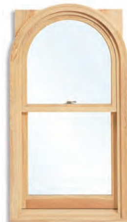
Round Top 6 Standard Double Hung with a round top appearance from the exterior, thanks to curved exterior components. Interior has a standard frame with rectangular sash and radius glass.*
