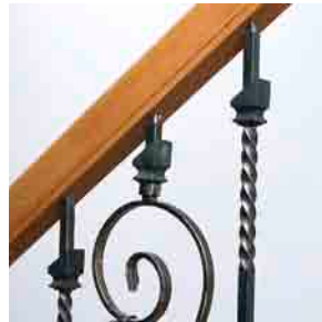
Step 5: Apply construction adhesive in the predrilled holes in the handrail. Position the handrail on top of the balusters. If top bases are being used, place one on each baluster before placing the handrail on top.
